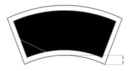
Min size of cut piece Min tolerance Larger items 200x100mm +/- 3mm +/- 5mm per m
